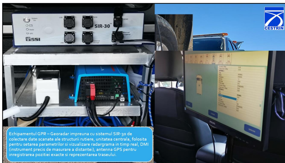
Echipament GPR/Sistem SIR-30
